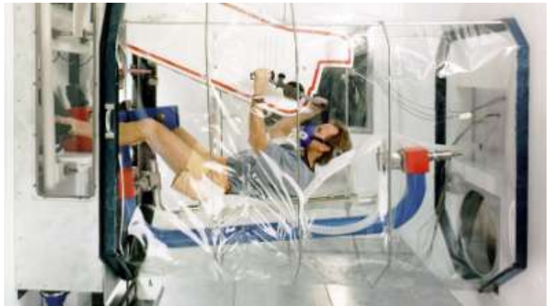
The EVA (Extra Vehicular Activity) Exercise Device is used to test potential astronauts on their weightlessness in space. It's housed at the NASA Ames Research Center in Mountain View, California. Photo: NASA
